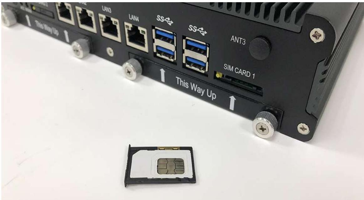
**Step 4.** Take the SIM card holder and Insert it into the socket as shown in the picture.
