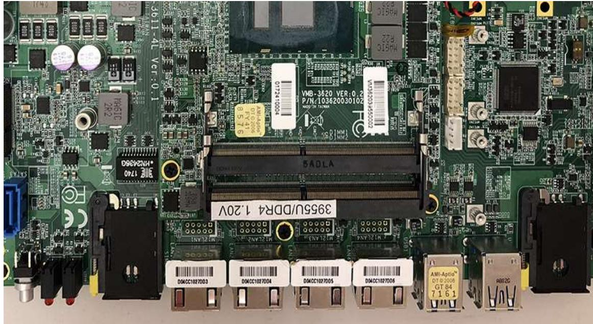
**Step2.** Hold the Memory with its notch aligned with the Memory socket of the board and insert it at a 30-degree angle into the socket as shown in the picture.
