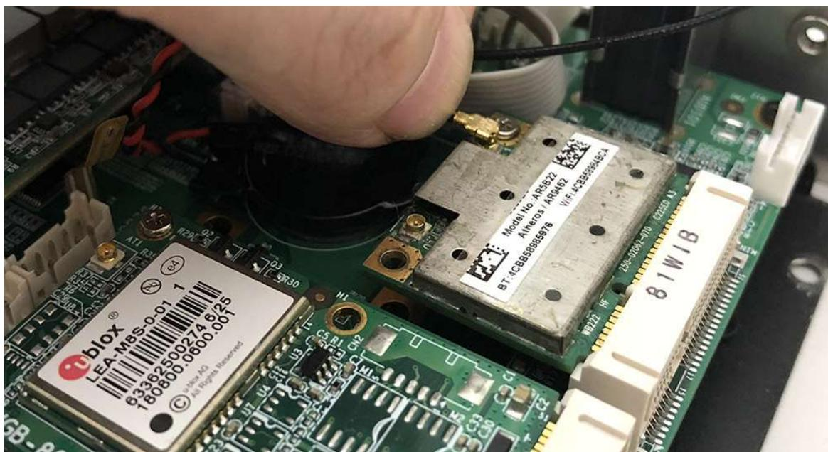
**Step 6.** Take the IpeX Connector and press on the 3G module as shown in the picture.
