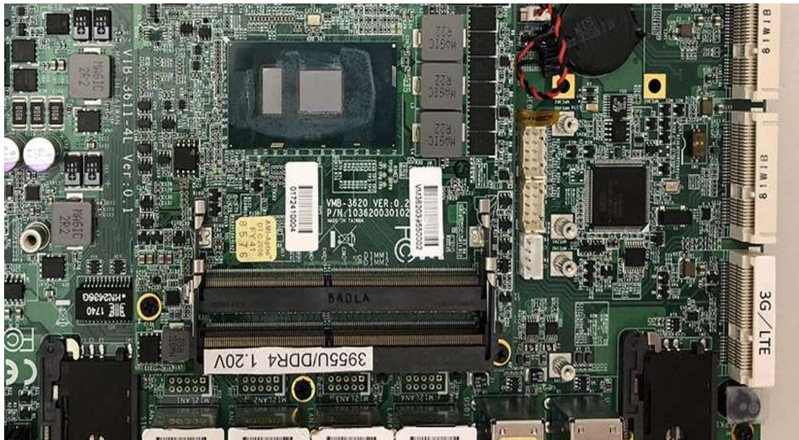
**Step 2.** Hold the Module with its notch aligned with the socket of the board and insert it at a 30 degree angle into the socket as shown in the picture.
