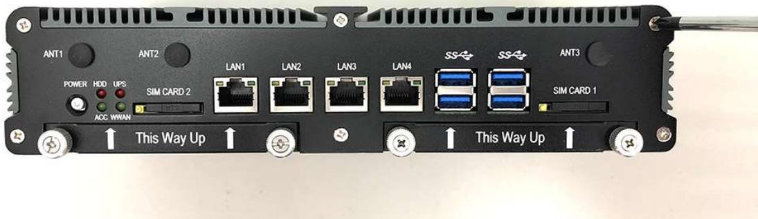
**Step3.** Unscrew the six screws of the Rear Panel as shown in the picture.
