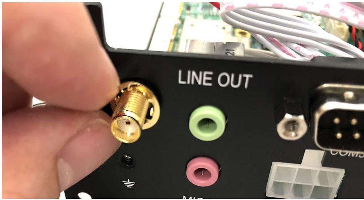
**Step 3.** Put the Oring to SMA Connector and tighten as shown in the picture.
