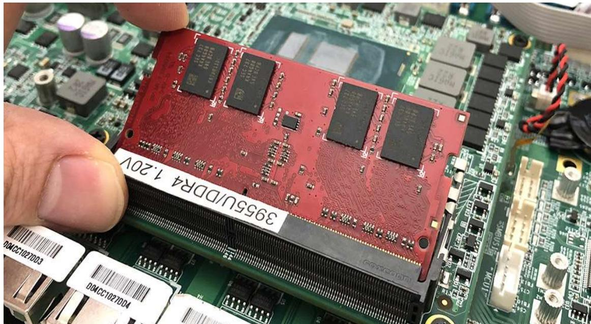
**Step3.** Press down on the Memory so that the tabs of the socket lock on both sides of the module as shown in the picture.
