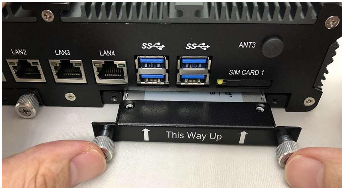
**Step 4.** Fully insert the HDD Holder into the socket until a “click” is heard as shown in the picture.
