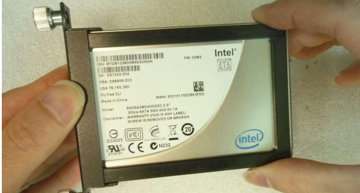
**Step 2.** Screw two screws on both side as shown in the picture.
