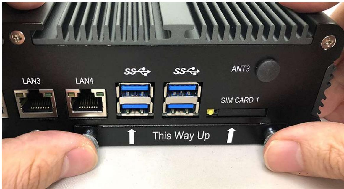
**Step 5.** Tighten to Storage Bracket screws as shown in the picture.
