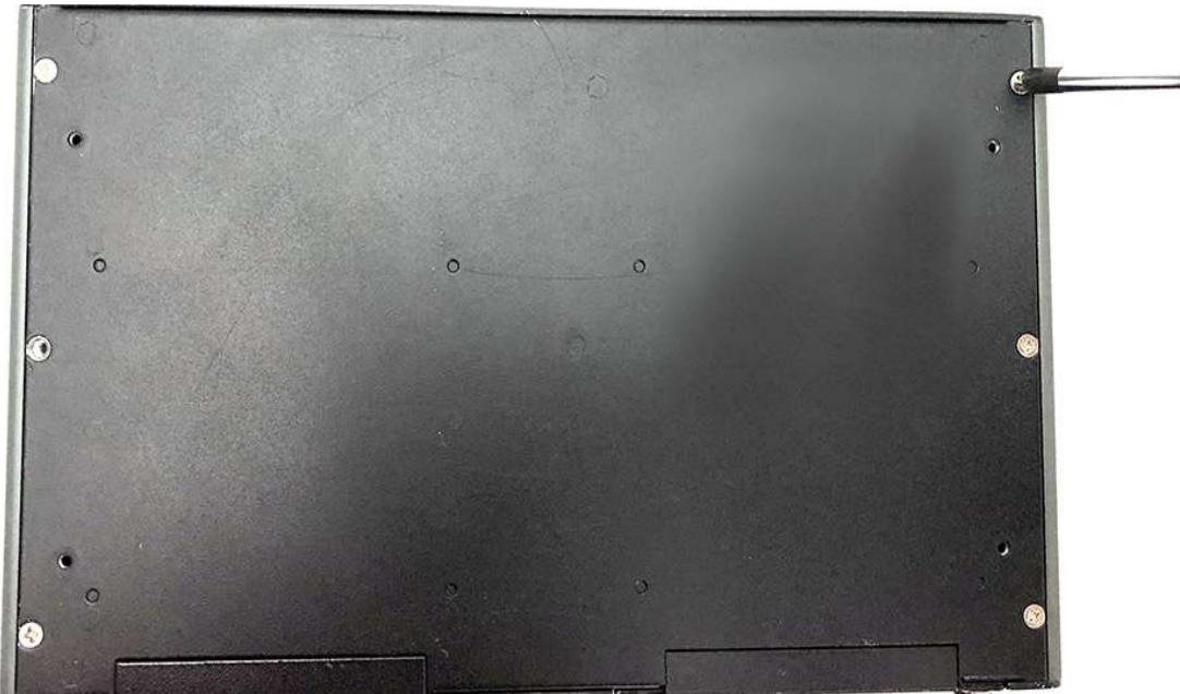
**Step2.** Unscrew the six screws of the Front Panel as shown in the picture.
