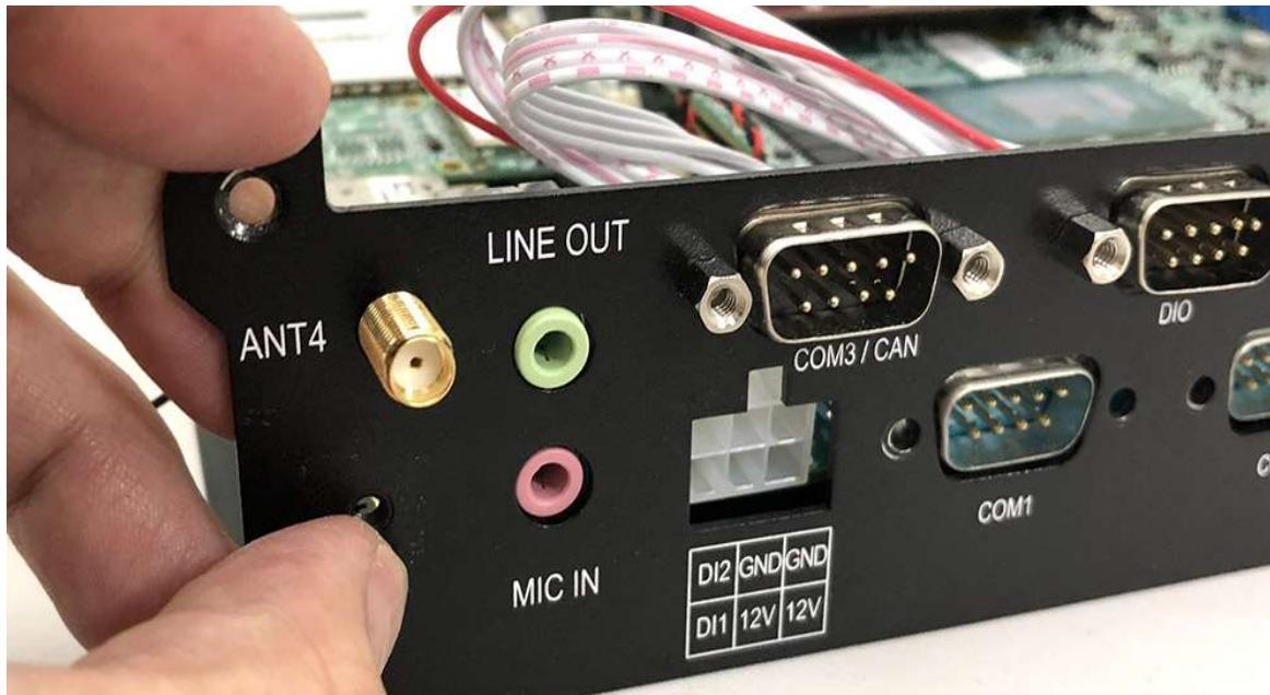
**Step 2.** Put the Washer into the SMA Connector as shown in the picture.
