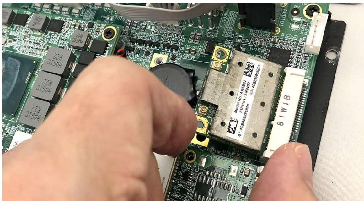
**Step 3.** Screwvone screw to the holder as shown in the picture.
