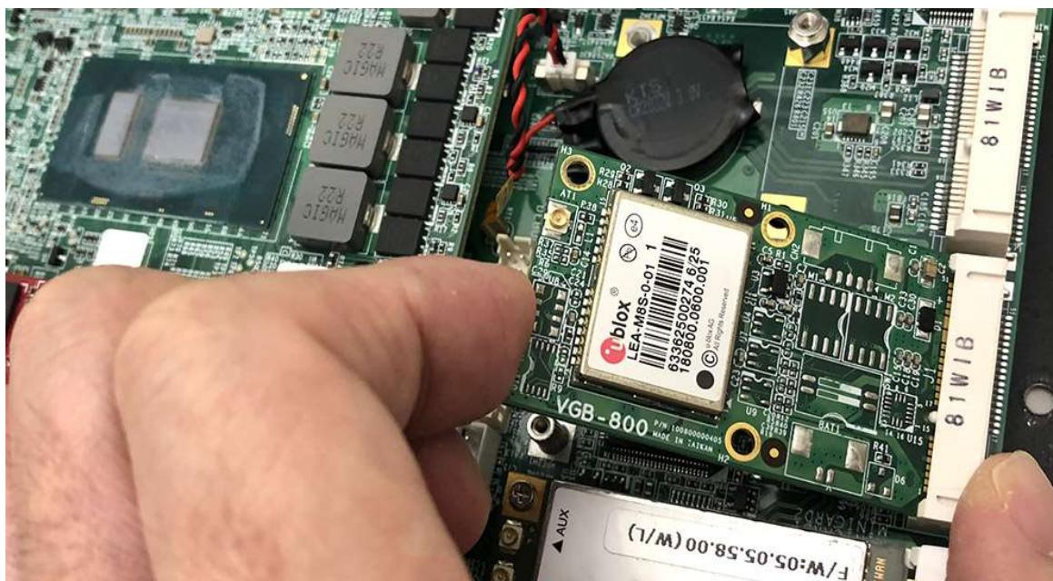
**Step 3.** Screw one screw to the holder as shown in the picture.
