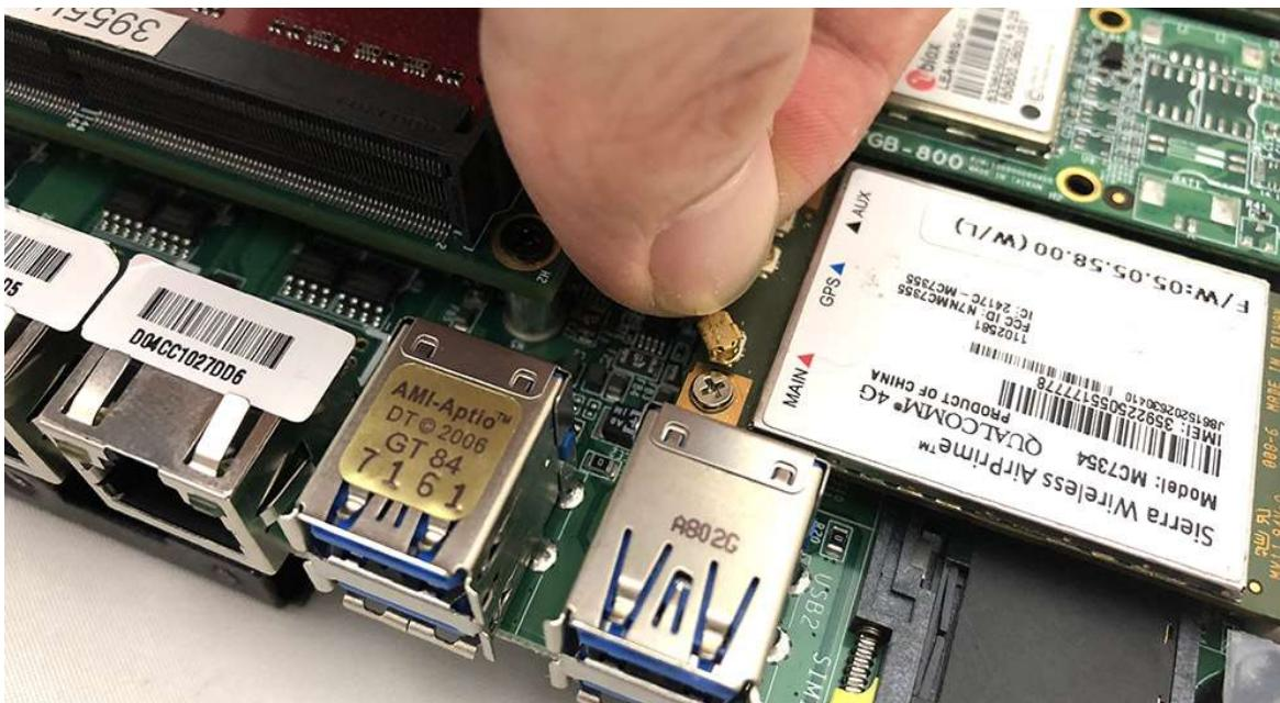
**Step 7.** Take the Ipeix Connector and press on the GPS module as shown in the picture.
