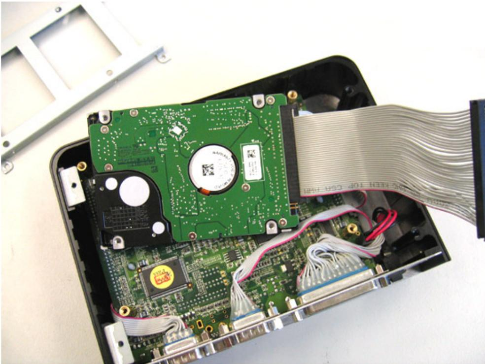
The 4 screws of the HDD are needed to install the HDD onto the mounting unit:
