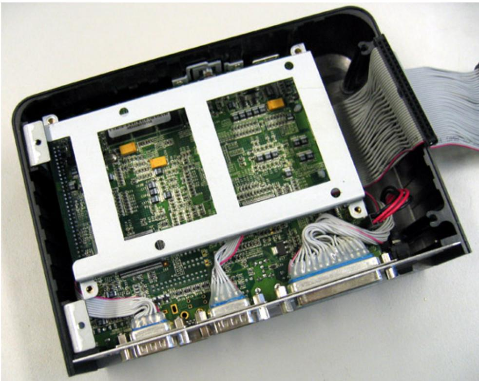
The HDD gets connected to the IDE cable, like shown in the picture:
