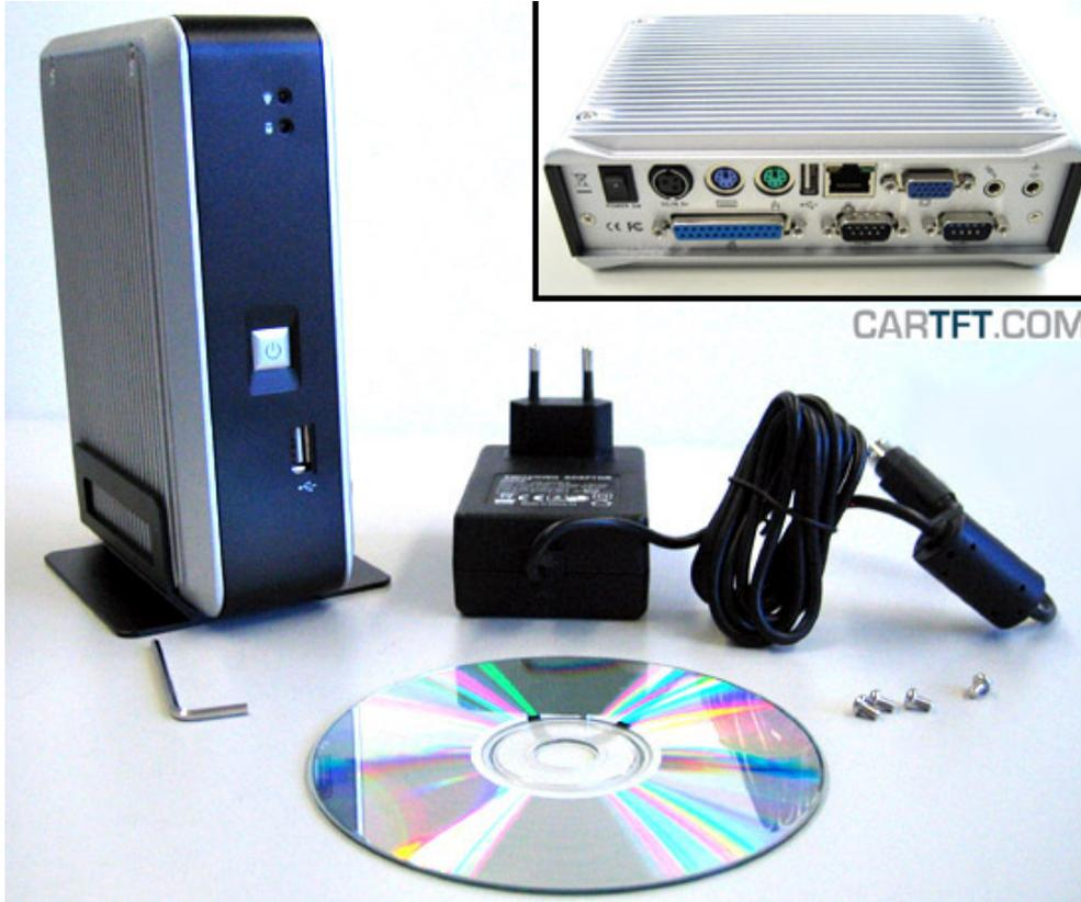
Open the socket head screws with the L-shaped hexagon key at the side, where the COM ports and also the parallel port are the nearest:
