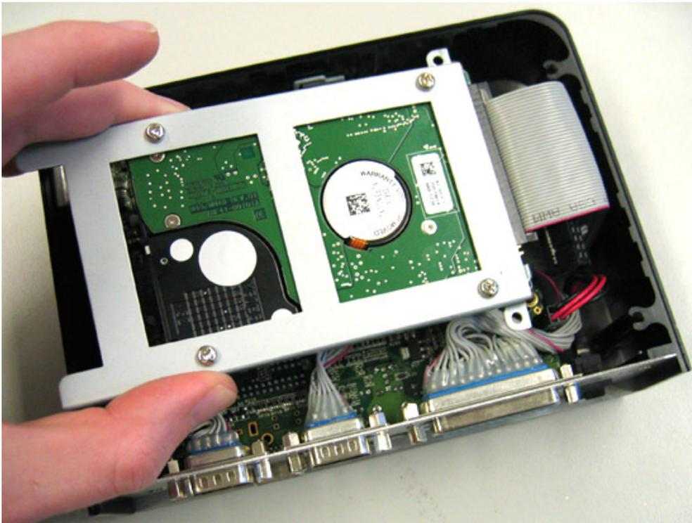
Install the HDD mounting unit into the enclosure again:
