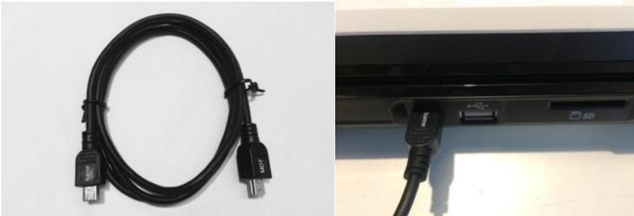
2. Plug the other end of the special USB cable with marked “MDT” to the CTFPND-9 cradle
