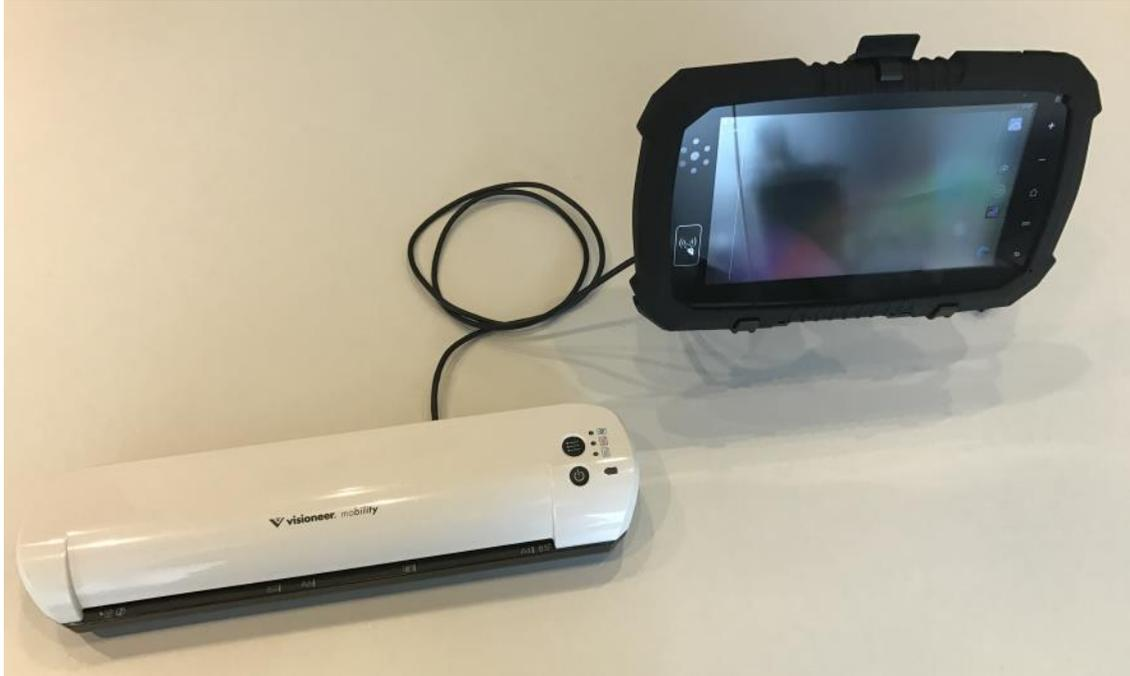
1. Plug the special USB cable with marked “scanner” to the mini USB port of the scanner.
