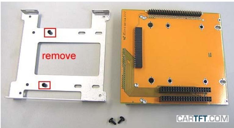
The HDD gets mounted onto the Drive Adapter:
