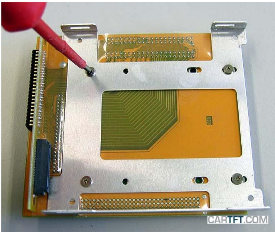
Install the two plastic spacers to the CD-ROM Adapter:
