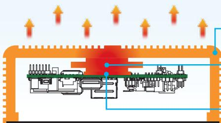
all aluminium body for quick heat dissipation
